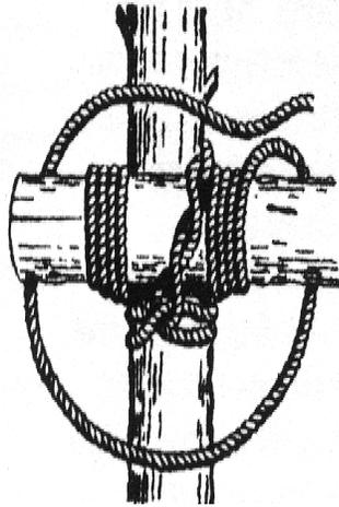
spars cross at an angle and touch each other. around the upright just below the crossing standing part around each other to secure the the horizontal spar, then behind the upright four times and end with a clove hitch on the
