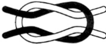
most common knot for joining two ropes. secure and reliable except when joining
