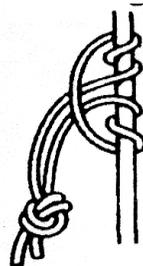
for attaching a small rope to a larger one. The smaller can be four, six or eight times.
